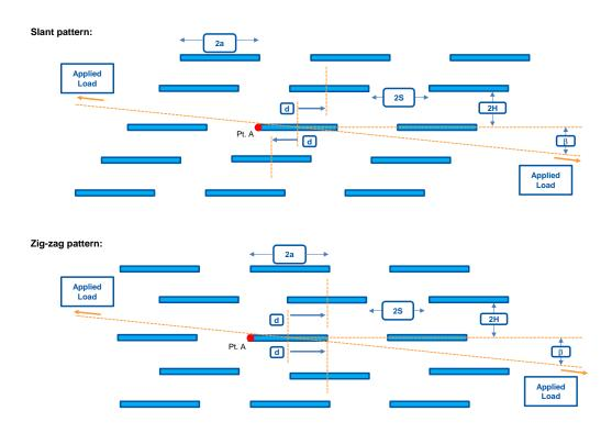
A group of 5 by 5 (25 in total) equally-sized flaws in various configurations was assessed. Two flaw patterns were investigated, slant and zig-zag (see Figure above). Four intra-row (within a single row) flaw spacings (S/a) were investigated: 0.5, 1.0, 1.5, and 2.0. For each intra-row spacing several inter-row shifts (d/a) were investigated that span the entire range of possible shifts.
