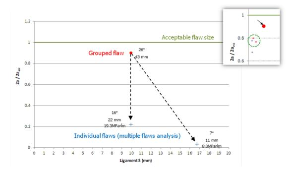
Similar 3D calculations were performed for the most critical isolated flaw, with similar results. The potential lack of conservativeness due to the neglected influence of the surrounding flaws on the calculated flaw, was largely compensated for by the over-conservativeness of the flaw grouping methodology.
