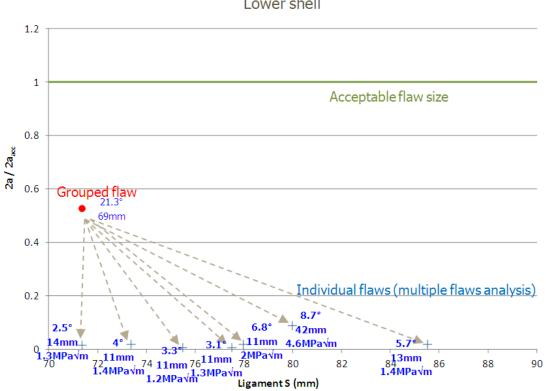
The results of such 3D calculations for the 7 ungrouped flaws show a significant increase of the margin with respect to the maximum allowable size.
