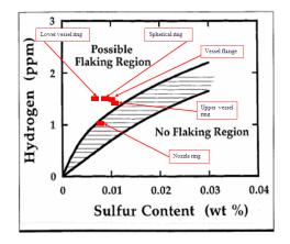
Although the chart above (R. J. Fruehan, *Iron & Steelmaker*, 1997)—adapted to the specificities of the Doel 3 RPV—is mainly indicative, both the upper and lower shells of the Doel 3 RPV shell are in the possible flaking region. The lower shell of the Doel 3 RPV, which is most affected by flakes, appears in the deepest part of this region.
